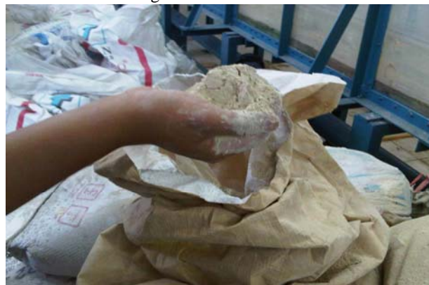
Fig. 3 Bentonite for scouring countermeasure
