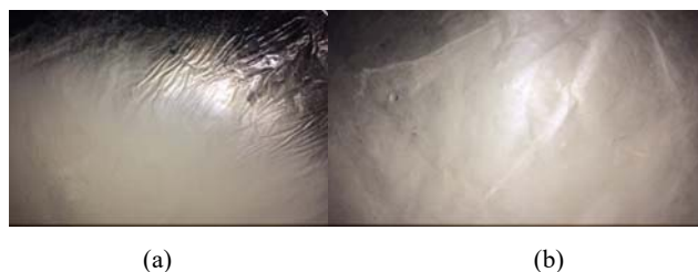
Fig. 3 PAN fibers using (a) Flat plate collector and (b) Drum Plate Collector
