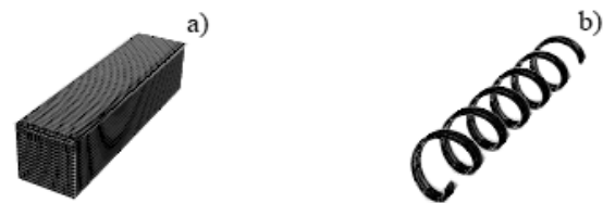
Fig. 5 Finite element triangulation (general quantity of elements 137738) (a) Finite element mesh of matrix, element type C3D4E, element quantity - 128873 (b) Finite element mesh of inclusion, element type C3D4E, element quantity - 8865 (Simulia Abaqus triangulation)
