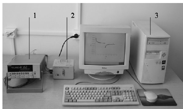
Fig. 2 Experimental setup for absorption/resorption currents measurement: 1 – Electrometer Keithley 6517, 2 – Resistivity Test Fixture Keithley 8009, 3 – PC
