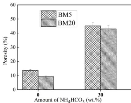
Fig. 3 Effect of  $\text{NH}_4\text{HCO}_3$  of  $\text{NH}_4\text{HCO}_3$  on porosity of sintered Ti-20Nb-5Ag alloys for BM5 and BM20
