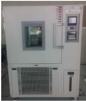
Fig. 3 Environmental (temperature) chamber used for the test
