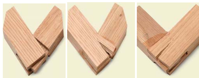
(a) Glue failure (b) Wood failure (c) Combination
