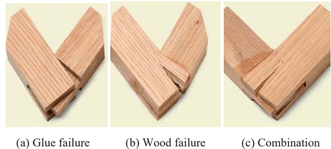
Fig. 1 Types of joints failure [6]
