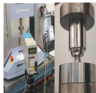
Fig. 4 Test setup of the Push-in assembly used for force application of the ball head against the stem
