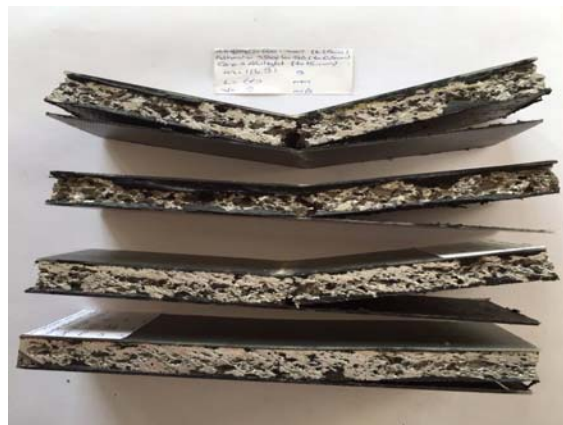
Fig. 9 Collapsed sandwiches named S1.5A15 after the bending tests at different support span values (top to bottom: L = 55, 70, 80 and 125 mm)
