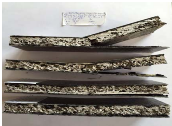
Fig. 7 Collapsed sandwiches named E1.5A15 after the bending tests at different support span values (top to bottom: L = 55, 70, 80 and 125 mm)
