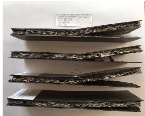
Fig. 8 Collapsed sandwiches named S1.5A10 after the bending tests at different support span values (top to bottom: L = 55, 70, 80 and 125 mm)
