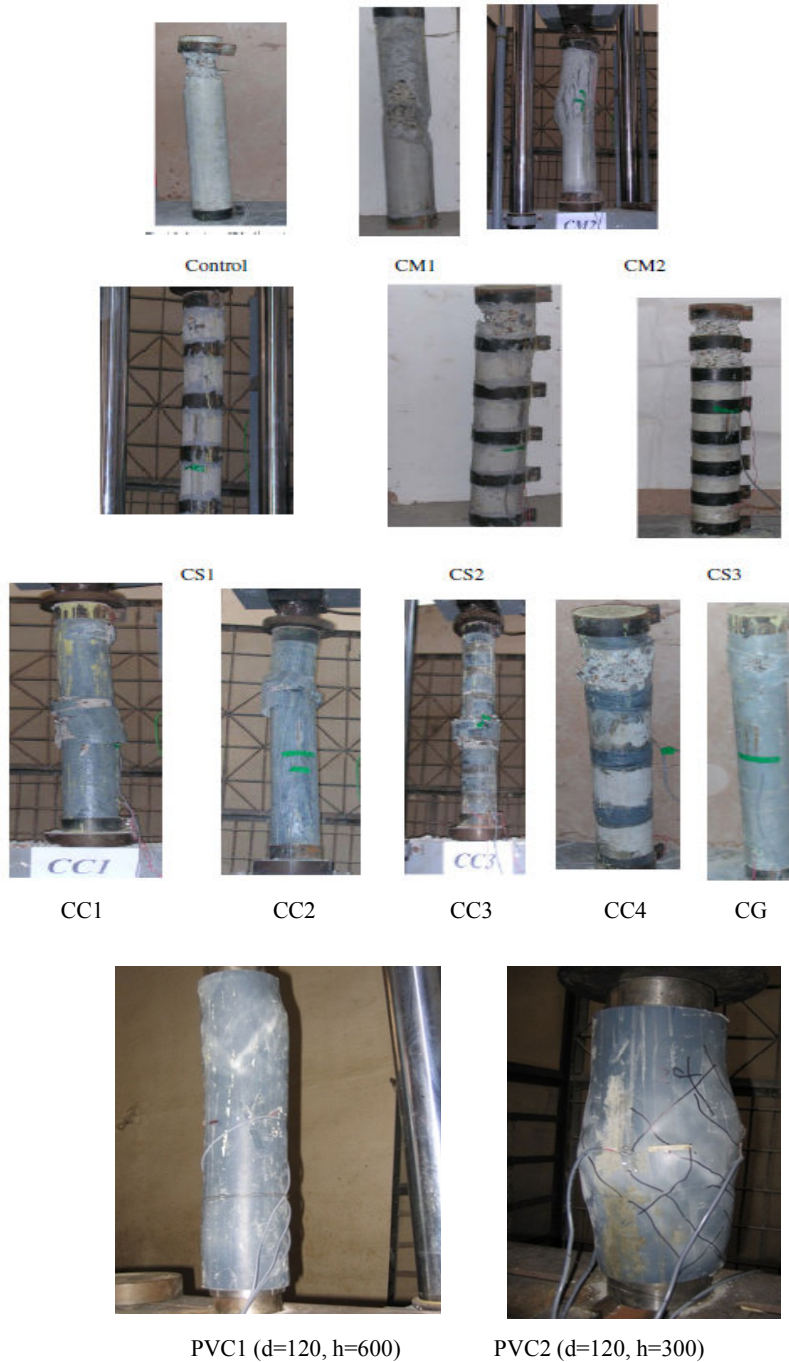
Fig. 2 Failure mode of tested specimens for confined columns
