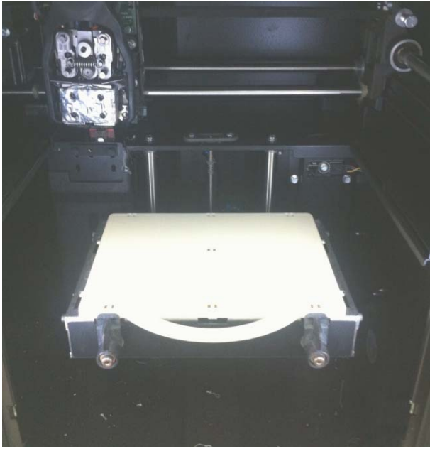
Fig. 8 Size verification of the modeling platform fabricated using the uPrint RP system
