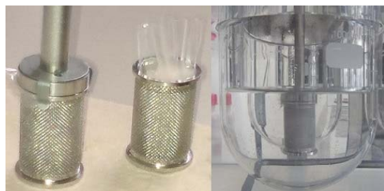
Fig. 2 Setup of the release test using dialysis tube and dissolution tester
