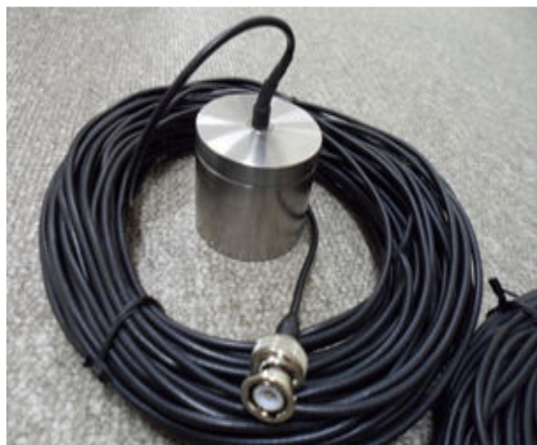
Fig. 5 Ultrasonic Sensor after waterproof
