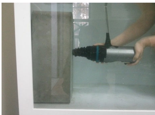
Fig. 6 Rebound Hardness Test in under water condition
