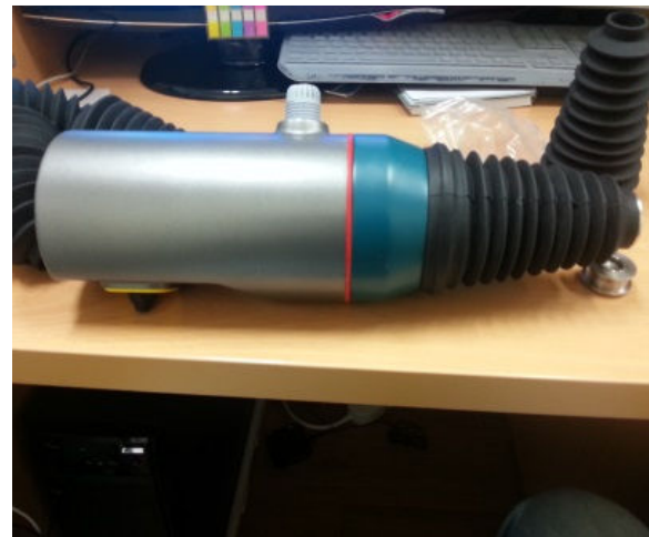
Fig. 2 Schmidt hammer after waterproof
