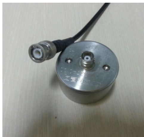
Fig. 4 Ultrasonic Sensor before waterproof
