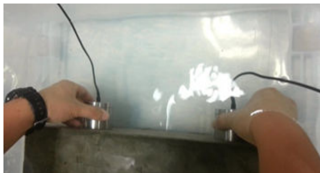
Fig. 7 Ultrasonic pulse velocity test in under water condition
