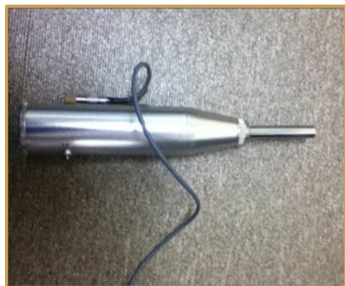
Fig. 1 Schmidt hammer before waterproof
