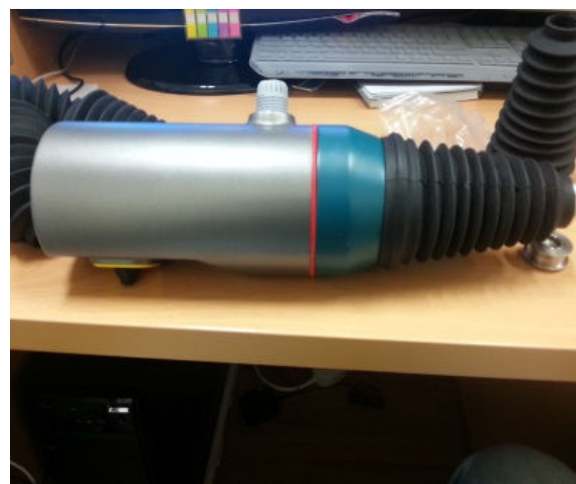
Fig. 2 Schmidt hammer after waterproof
