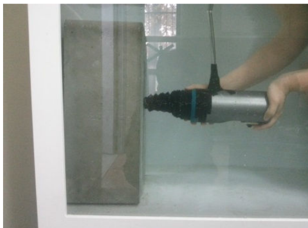
Fig. 6 Rebound Hardness Test in under water condition
