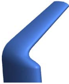
Fig. 11: Geometry of the first analyzed winglet
