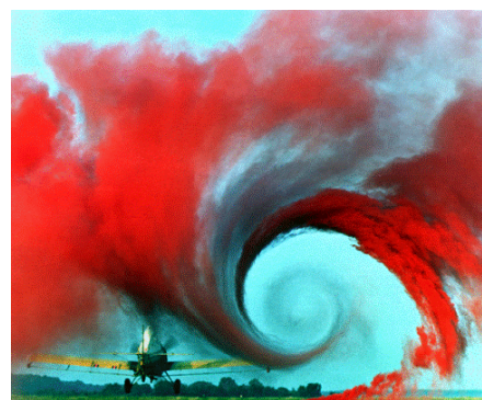
Fig. 2: Tip vortex rolling up from a wingtip (from: [4])
