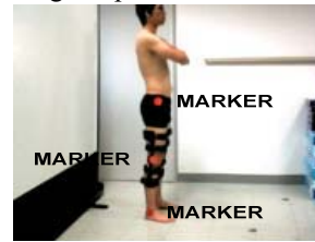
Fig.3 Location of the markers and approximation of model using a 5-link biped model
