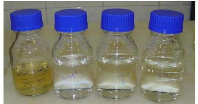
Fig. 5 Quality of sample in inlet and outlet of resin and carbon active beds(left. 1st, polluted amine right, 2st to4rd batch of outlet bed)
