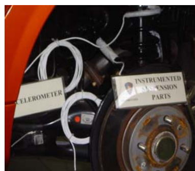
Fig. 2 Instrumented suspension system
