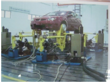
Fig. 3 MTS 320 multi-axial spindle coupled road simulator
