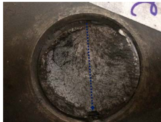
Fig. 9 Fracture of pin 2 due to bending overload stress generating brittle fracture (radial marks). The blue dotted arrow indicates the direction of instantaneous propagation
