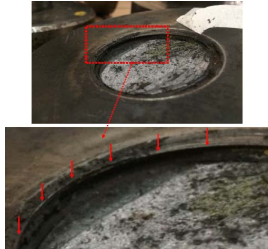
Fig. 8 Presence of sharp edge (sharp corners) in the peaks of the threads of the seat of the fracture pin 1
