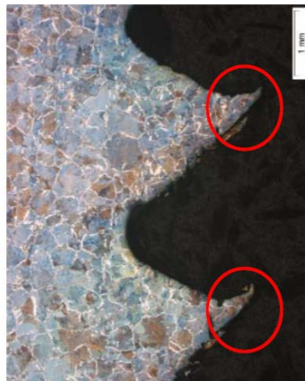
Fig. 10 The presence of a sharp edge in the peaks of the threads of the seat of the fracture pin 1
