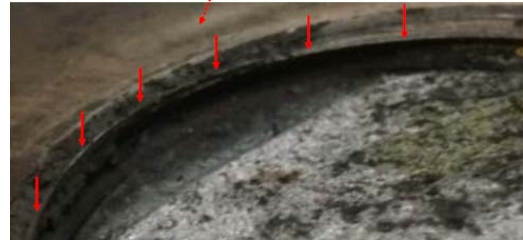
Fig. 8 Presence of sharp edge (sharp corners) in the peaks of the threads of the seat of the fracture pin 1
