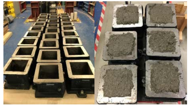
Fig. 4 Steel Cube Moulds used to Cast Concrete Specimens
