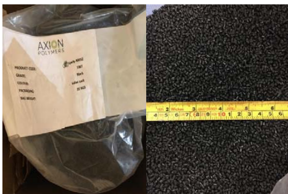
Fig. 3 Plastic Aggregate Material
