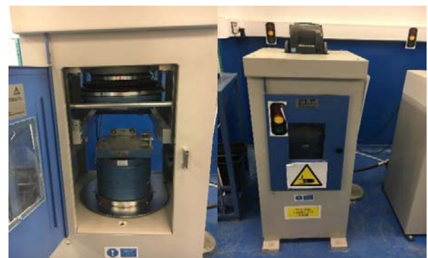
Fig. 5 Compressive Strength Testing Machine
