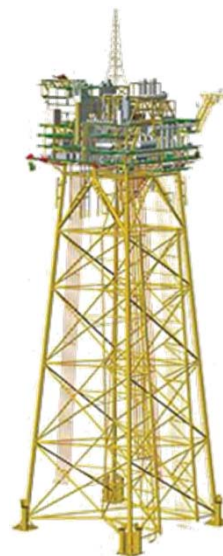
Fig. 1 Typical Jacket Platform (adapted from offshore-technology.com)
