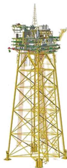
Fig. 1 Typical Jacket Platform (adapted from offshore-technology.com)
