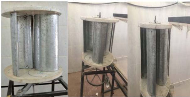
(a) Two blades (b) Three blades (c) Four blades
