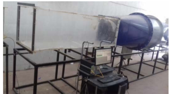
Fig. 2 Wind tunnel used for flow generation
