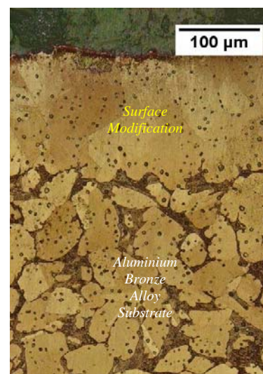
Fig. 2 Polarised light microscopy image of surface modification on Al bronze alloy after modified surface
