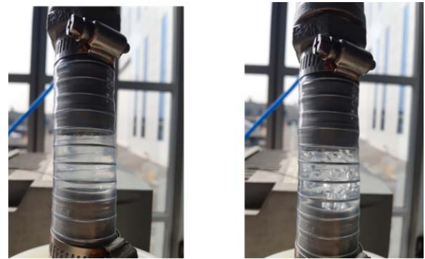
(a) at low flow rate of gases (b) at high flow rate of gases
