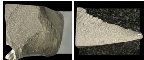
Fig. 13 Fracture of carbide bit
