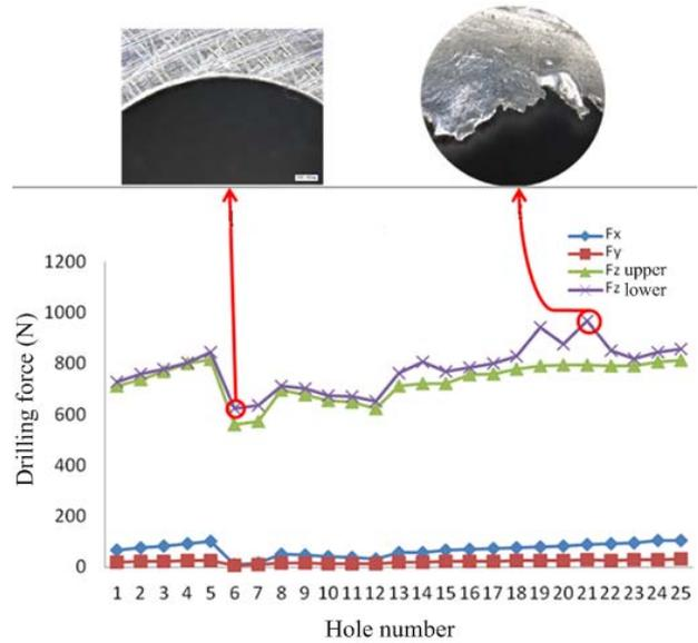
Fig. 15 Change of drilling force when the HSS tool was used
