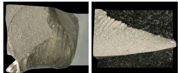
Fig. 13 Fracture of carbide bit
