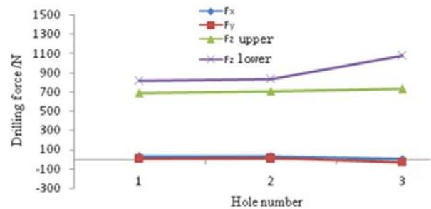
Fig. 16 Change of drilling force when the carbide tool was used
