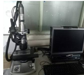
Fig. 3 VHX-1000C digital stereo Microscope
