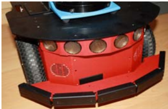
Fig. 3 Pioneer P3DX fitted with the Polaroid Sonar Array (front and rear) and a Bumper Array at the front
