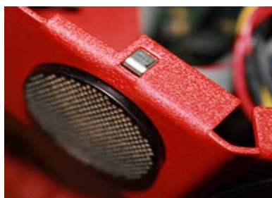
Fig. 4 Polaroid Sonar Sensor Transducer is used for operations in air at ultrasonic frequencies
