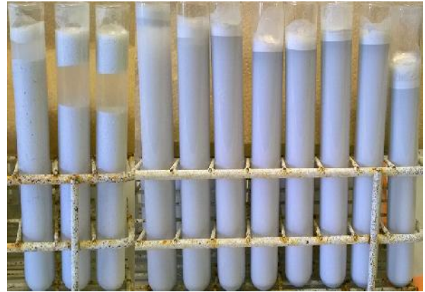
Fig. 11 Samples at 0.015 wt.% SDBS and different pH values, from left to right: pH=6.4 - 6.6 - 7.1 - 6 - 5.8 - 5.6 - 5.4 - 5.2 - 4.9 - 4.5 - 3.9
