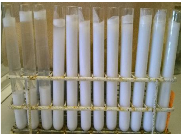
Fig. 10 Samples at 0.01 wt.% SDBS and different pH values, from left to right: pH=7.2 - 6.9 - 6.5 - 6.3 - 5.9 - 5.6 - 5.3 - 5 - 4.8 - 4.5 - 4.2 - 4
