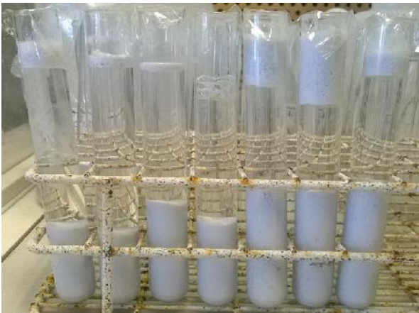
Fig. 9 Samples at 0.1 wt.% SDBS and different pH values, from left to right: pH=8 - 9.3 - 10 - 10.7 - 11.4 - 2 - 2.6 - 3
