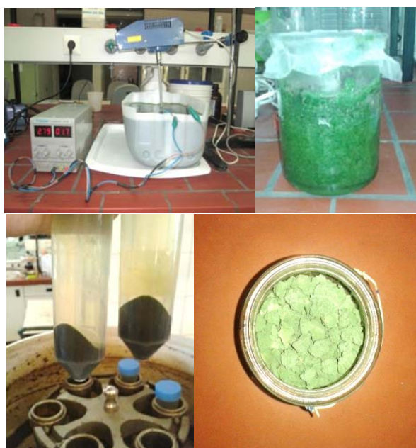
Fig. 3 Microalgae harvesting, desalinating and drying
