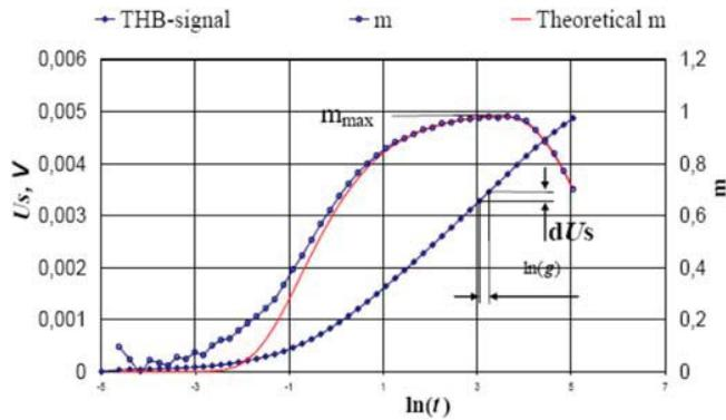
Fig. 2 Typical response of THB sensor [24]
