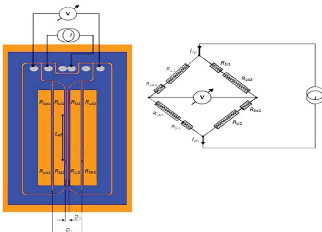
Fig. 1 THB6K sensor and equivalent electrical circuit diagram [24]
