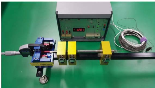
Fig. 7 Experiment for fuel stack elongation measurement
