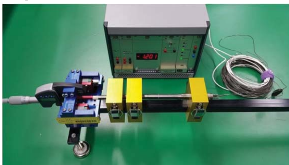
Fig. 7 Experiment for fuel stack elongation measurement
