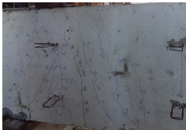
(a) Typical shear crack patterns for panel GS5 along the height of the concrete wythe
