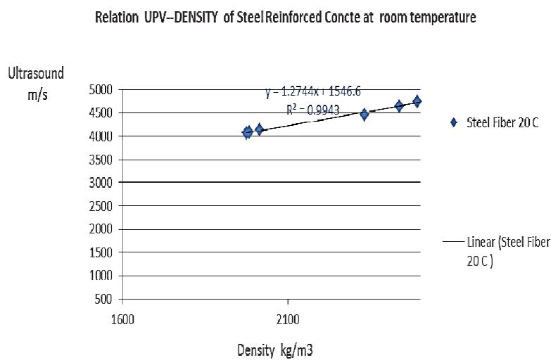
Fig. 6 Relation UPV-Density of Steel Reinforced Concrete at room temperature
