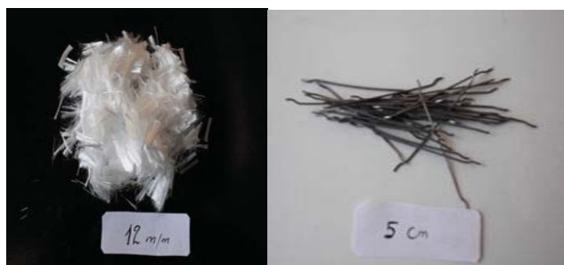
Fig. 3 Polypropylene of length 12 mm and Steel Fiber of length 5 cm
