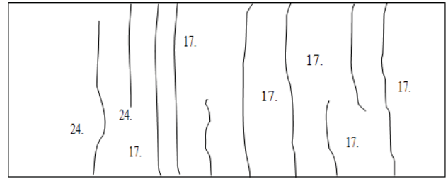
(a) Typical crack pattern for panel as one-way slab – bottom wythe
