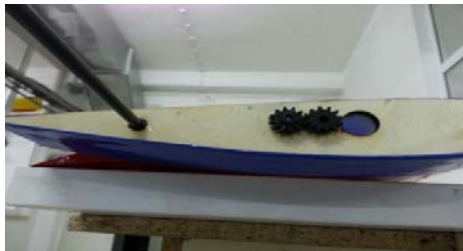
Fig. 7 Placement of the Servo Motor in the Wing
