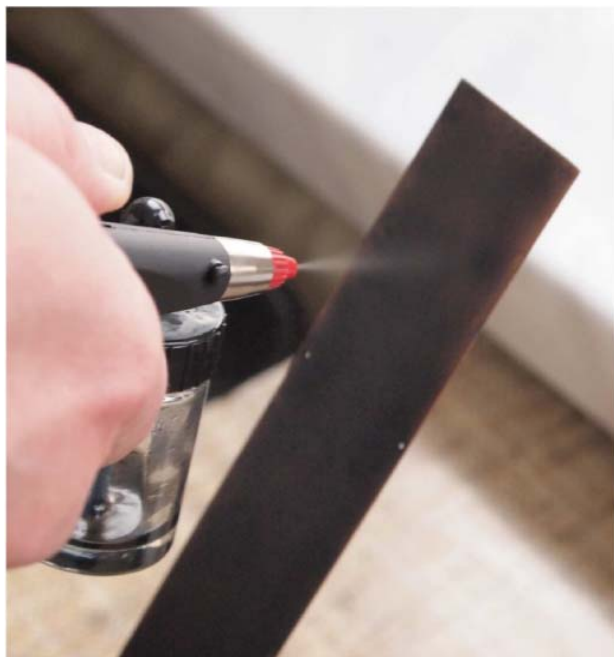
Fig. 5 Spreading carbon nanotubes with the airbrush [5]
