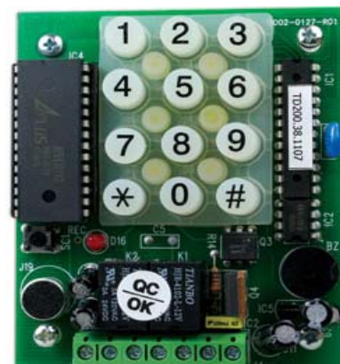
Fig. 3 The DTMF unit
