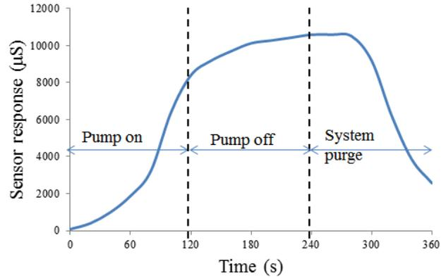
Fig. 6 A sample sensor response curve
