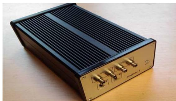
Fig. 1 DiagNose II e-nose system
